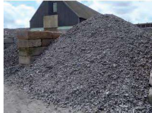
Non-Ferrous fraction 12-40 mm
